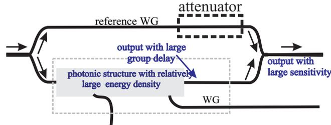
Fig. 3. Schematic of a MZI like set-up to convert partial group delay and sensitivity into each other.
