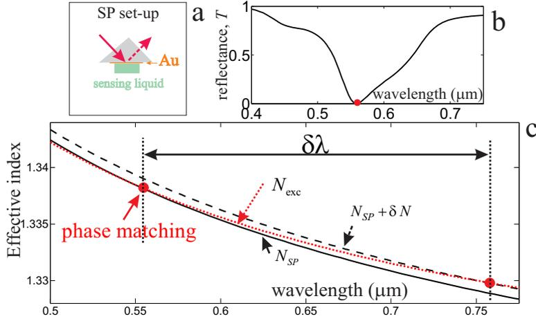
Fig. 1. Illustration of the huge spectral shifts in a SP set-up: a) schematic of the set-up, b) a typical response curve with  $R$  the reflectance, and c) idealized dispersion curves for the excitation (dotted line), the SP (solid line), and for the SP after a small modal index change  $\delta N$  (dashed line).
