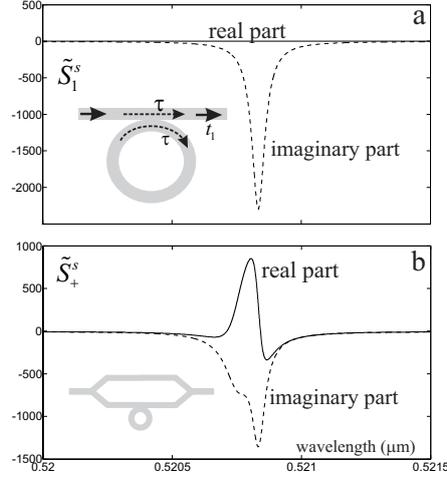
Fig. 4. Real and imaginary parts of the quantities  $\tilde{S}_1^s$  (a) and  $\tilde{S}_+^s$  (b) versus excitation wavelength. The insets show the considered structural lay-outs.
