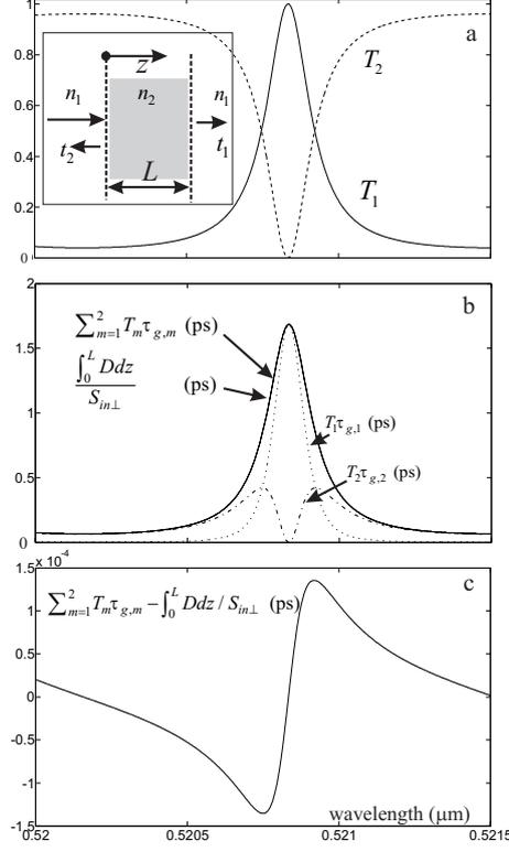
Fig. 2. Computational results for a simple Fabry-Perot cavity: a) schematic of the structure and reflectance  $T_2$  and transmittance  $T_1$ , b) and c) dispersion curves of the indicated quantities.
