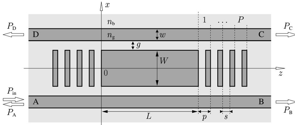
Fig. 1. Grating assisted rectangular resonator: Two parallel waveguide cores of width  $w$  are coupled by a cavity of width  $W$  and length  $L$ , separated by gaps  $g$ . Gratings with  $P$  periods of length  $p$  with a spacing  $s$  enclose the cavity. The guiding regions with refractive index  $n_g$  are embedded in a background medium with index  $n_b$ . Capital letters A to D denote the input and output ports.
