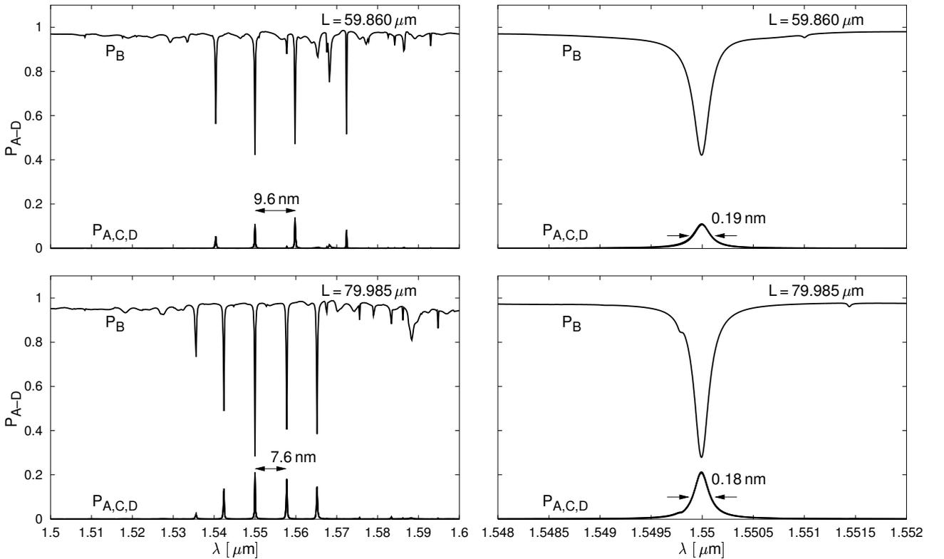
Fig. 3. Spectral responses of resonators according to Fig. 1, with the parameters of Table 1, for cavity lengths  $L = 59.860 \mu\text{m}$  (top) and  $L = 79.985 \mu\text{m}$  (bottom).  $P_A$  to  $P_D$  are the relative power fractions that are reflected or transmitted into ports A to D. The curves related to  $P_A$ ,  $P_C$ , and  $P_D$  are almost completely superimposed.
