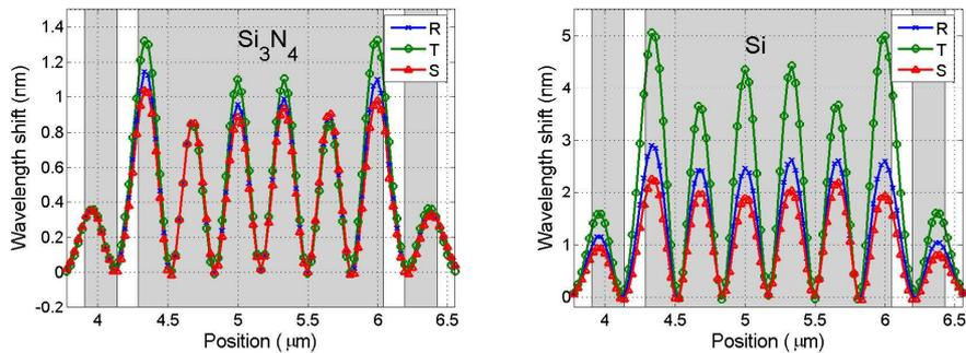
Figure 5: Estimated wavelength shift of the resonance for the silicon nitride (left) and silicon (right) tips; each line is the wavelength shift estimated by only considering the  $R$ ,  $T$  or  $S$  curve in Figure 4. Note the different scales of the shifts in the two graphs.
