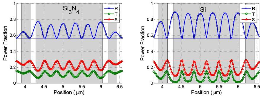
Figure 4: Reflected, transmitted and scattered power as a silicon nitride (left) or silicon (right) tip is scanned over the surface around the central defect (gray patches: high index regions). The horizontal lines denote the values without the tip.
