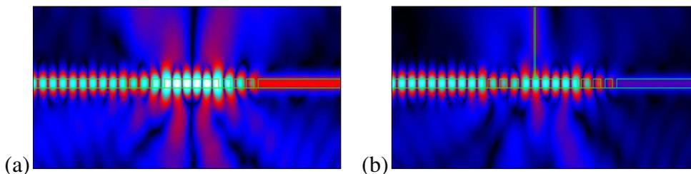
Figure 3: Logarithm of absolute value of the principle dielectric component of the field in the defect grating at a wavelength of  $1.734 \mu\text{m}$ . a: without tip; b: with silicon tip
