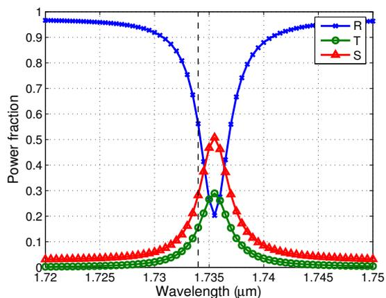
Figure 2: Spectrum of the structure of Figure 1 for unit input from the left;  $R$  is the reflected modal power,  $T$  is the transmitted modal power, and  $S$  is the scattered (lost) power.
