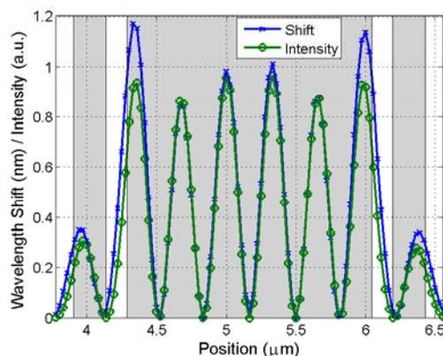
**Fig. 4** Estimated wavelength shift and optical intensity at the end of the tip
