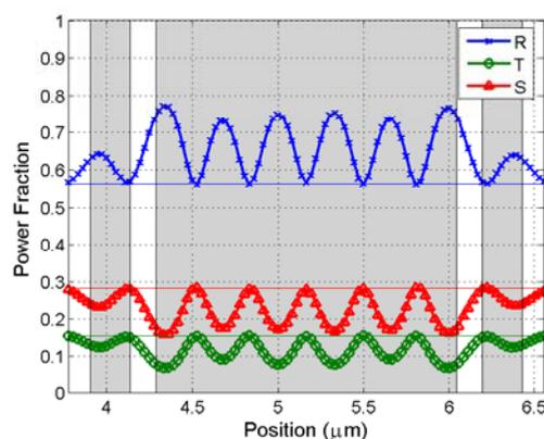
**Fig. 3** Powers as a function of nitride tip location
