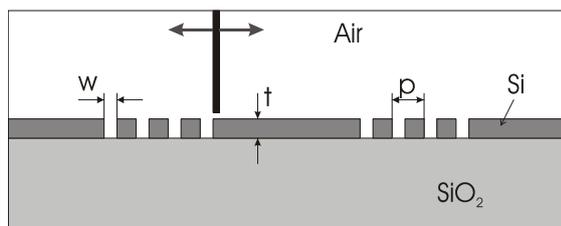
**Fig. 1** Silicon on Insulator defect grating structure under consideration. Refractive indices:  $\text{SiO}_2 - 1.45$ ,  $\text{Si} - 3.4$ ,  $\text{Air} - 1.0$ ,  $\text{Si}_3\text{N}_4 - 2.0$ . Grating period  $p = 380 \text{ nm}$ ; air hole width  $w = 150 \text{ nm}$ ; waveguide thickness  $t = 220 \text{ nm}$ .
