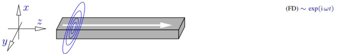
Longitudinally homogeneous waveguide: mirror symmetry  $z \rightarrow -z$ .
