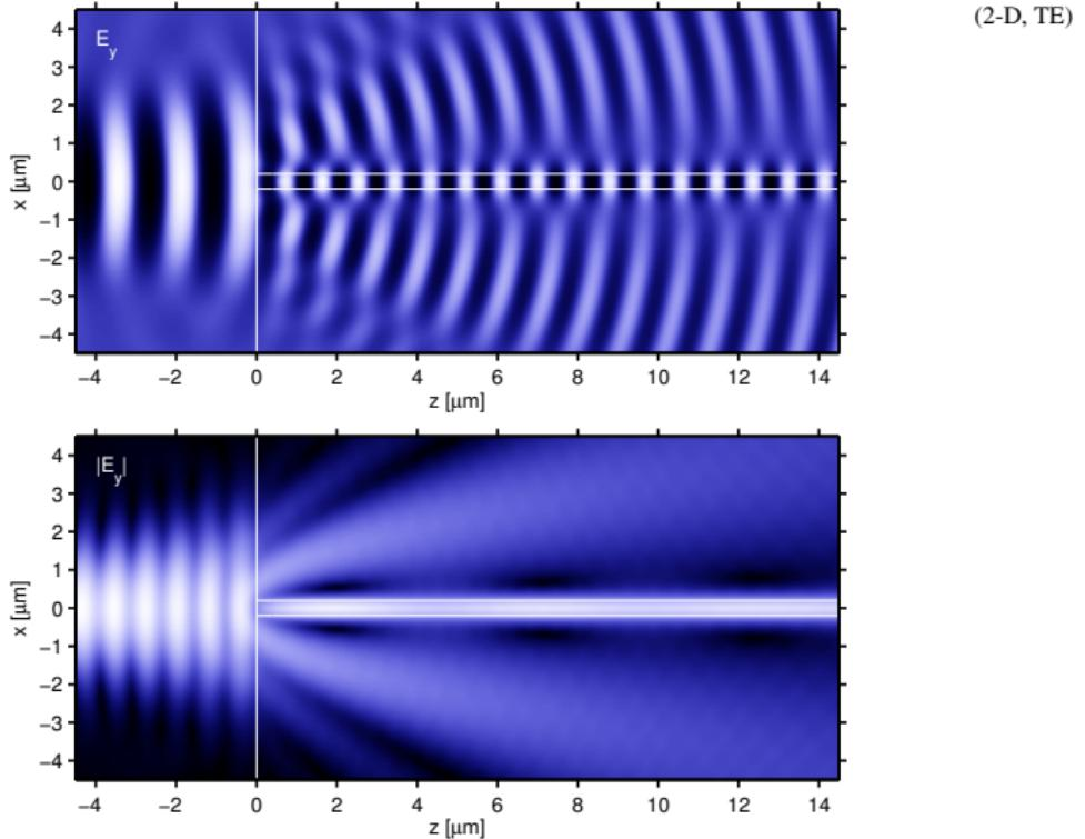
*Butt-coupling to a waveguide facet.*
