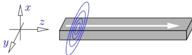
Unidirectional guided waves in a “long” dielectric channel that supports fundamental TE- and TM-like modes only:
