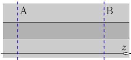
$\mathbf{E}, \mathbf{H}$ : a solution of the Maxwell equations for the  $z$ -homogeneous waveguide between two cross sectional planes A and B.
